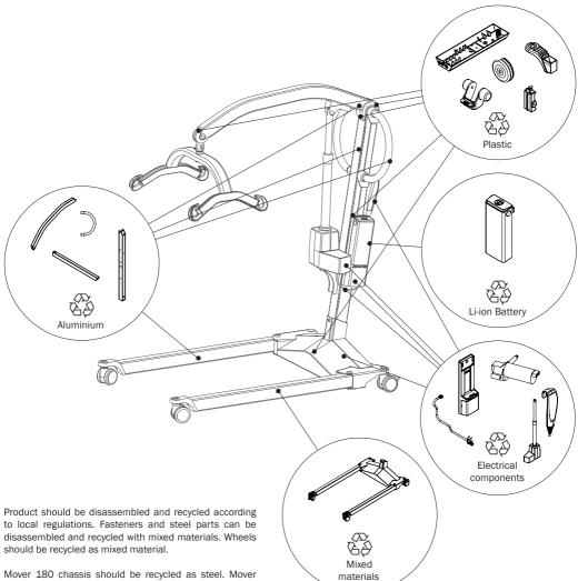
Mover 180 chassis should be recycled as steel. Mover 205/300 chassis should be recycled as aluminium. Wiring and cables should be recycled as electronics.
