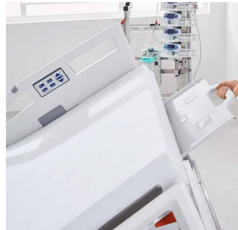
◀ Thanks to the radiolucent backrest and the integrated X-ray cassette holder, there is no need for time-consuming relocation of the patient.
