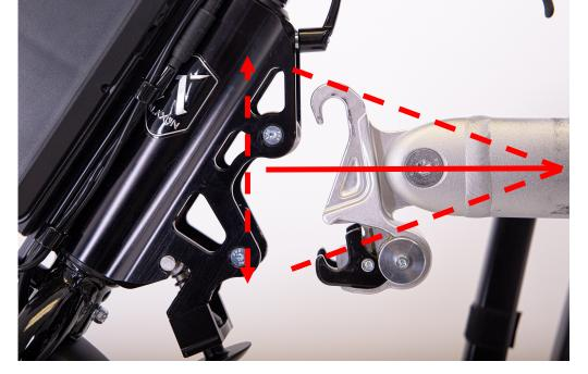
The upper hook of the KLICK connector should 4. fit to the upper pin and move freely over it. The distance between the lower hook on the KLICK connector and the lower pin located on the coupling plate must be 0,5 to 1 cm
