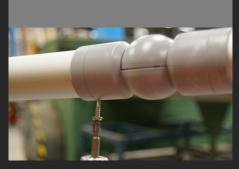
15. Mount the two included screws to fixate the rail link.
