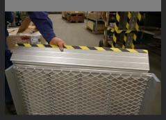
3. Mount the upper part (ÖL) in the slot on the upper half of the ramp. No screws needed! Put the ramp on existing platform
