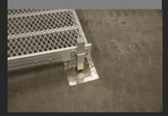
4. Mount support legs on both sides of the ramp. Plumb the legs and tighten the screws. Always tighten the left screw first
