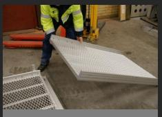
6. Lay down the next ramp section. Repeat 4–5 until desired length
